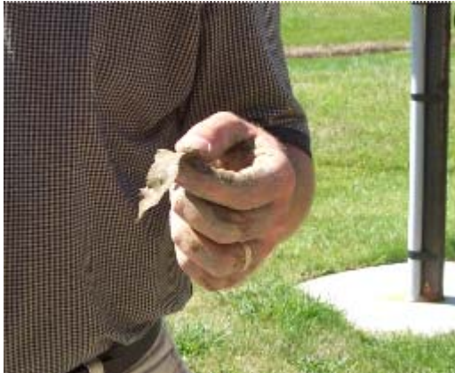
When soil will form a long, thin ribbon like the one pictured above, it is too wet to install a soil absorption system
