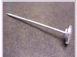
A typical metal stem dial thermometer. Note the calibration nut on the bottom
